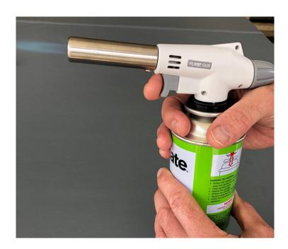
6. To turn off, simply rotate the grey valve clockwise until the gas stops flowing and the flame is extinguished:
