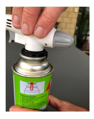
5. To ignite the Flame Torch, ensure the nozzle is pointed in a safe direction, rotate the grey valve counter-clockwise until you can hear a small amount of gas flowing and then squeeze the trigger:
