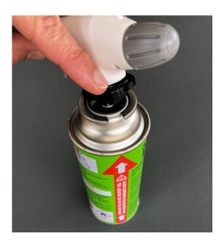
4. Press the Flame Torch down onto the Butane Cartridge and gently rotate the white body of the Flame Torch clockwise to connect the two:
