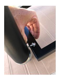
6. Once all bolts have been screwed in by hand, tighten all 4 bolts using a 7/16" or 11mm socket or spanner until the spring washer has been compressed. Do not overtighten otherwise the nylon washer will split, and you could damage the thread:
