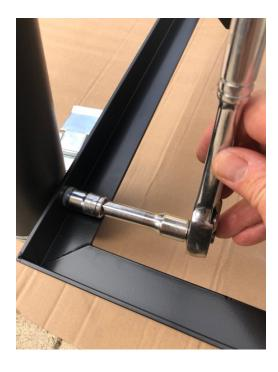
7. Re-tighten all 8 of the hex cap screws on the legs using a 5/32" or 4mm allen key:
